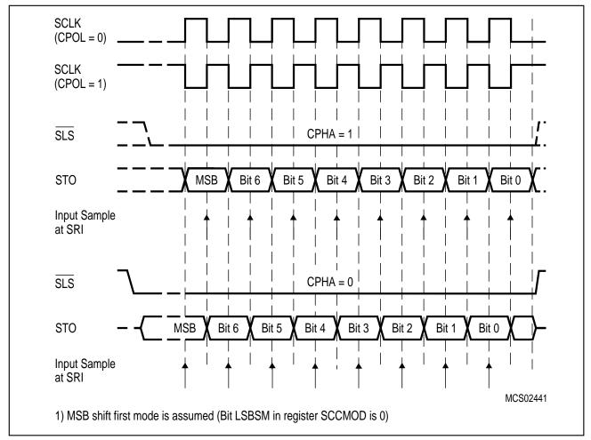
Figure 6-40 Slave Mode Operation of SSC
