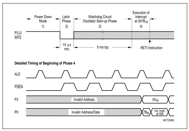
Figure 9-1 Wake-up from Power Down Mode Procedure
