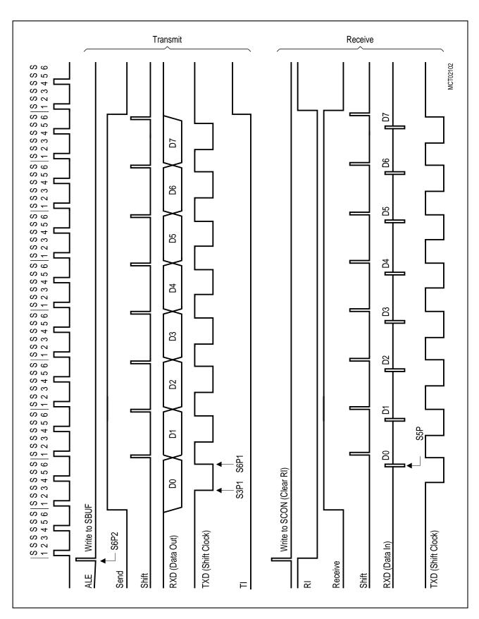
Figure 6-32 Serial Interface, Mode 0, Timing Diagram
