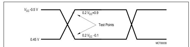
AC Inputs during testing are driven at  $V_{\rm CC}$  - 0.5 V for a logic '1' and 0.45 V for a logic '0'. Timing measurements are made at  $V_{\rm IHmin}$  for a logic '1' and  $V_{\rm ILmax}$  for a logic '0'.
