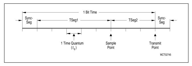
Figure 6-50 Bit Timing Definition
