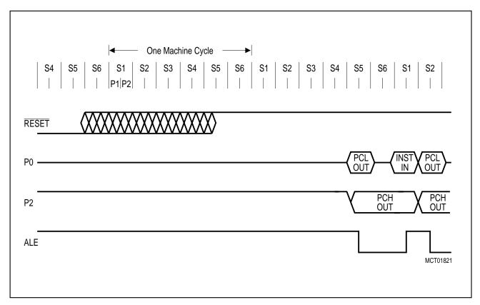
Figure 5-2 CPU Timing after Reset
