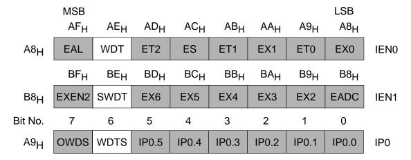
The shaded bits are not used for fail save control.
