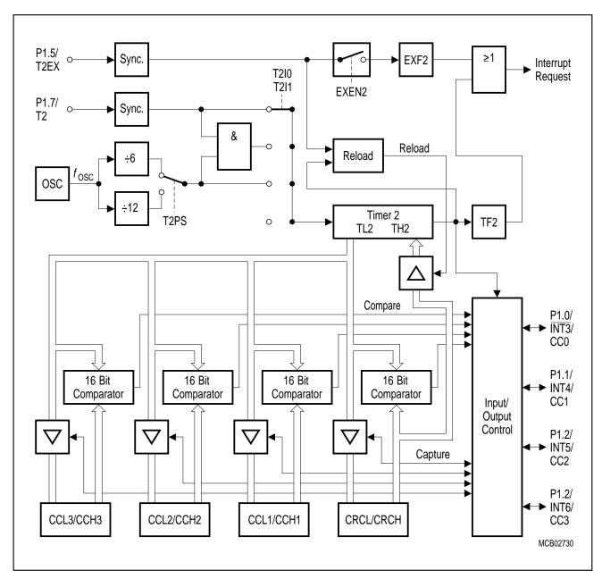
Figure 6-19 Timer 2 Block Diagram
