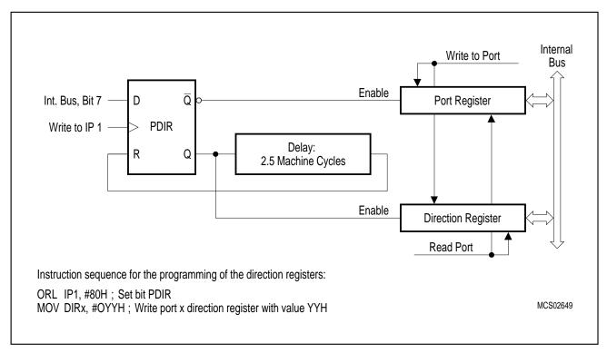
Figure 6-2 Port 5 Register, Direction Register
