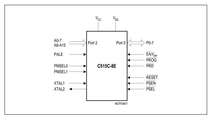
Figure 10-1 C515C-8E Programming Mode Configuration
