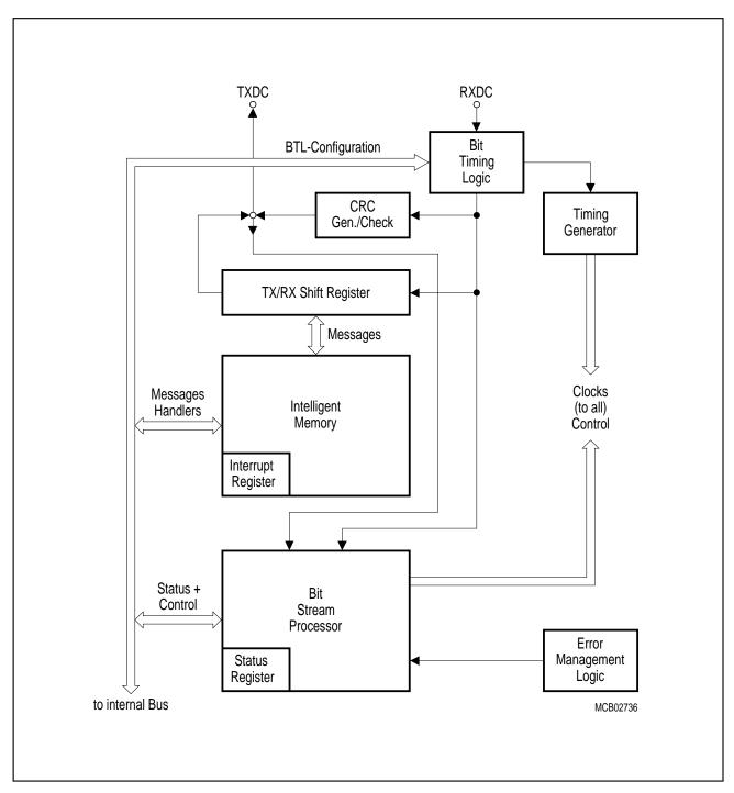
Figure 6-41 CAN Controller Block Diagram
