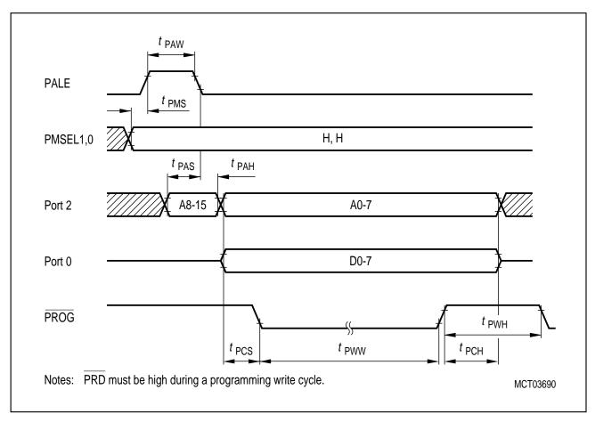
**Programming Code Byte - Write Cycle Timing**
