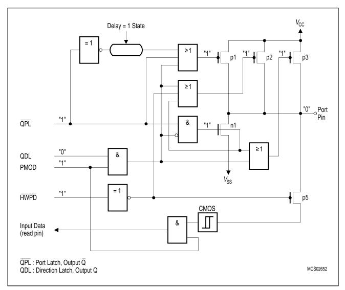
Figure 6-11 Bidirectional Port Structure - Output Mode - "0"
