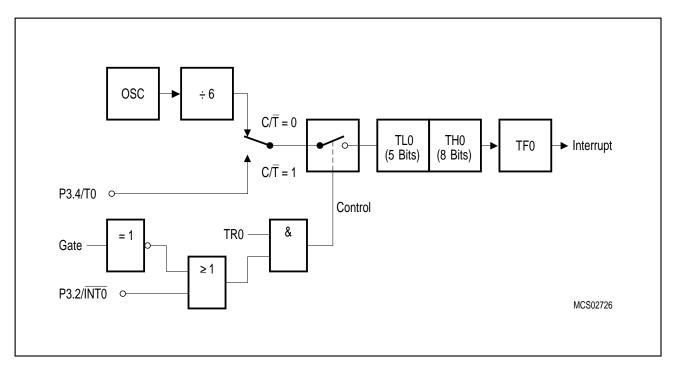
Figure 6-15 Timer/Counter 0, Mode 0: 13-Bit Timer/Counter
