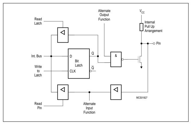
Figure 6-13 Circuitry of Ports 1, 3, 4 and 7
