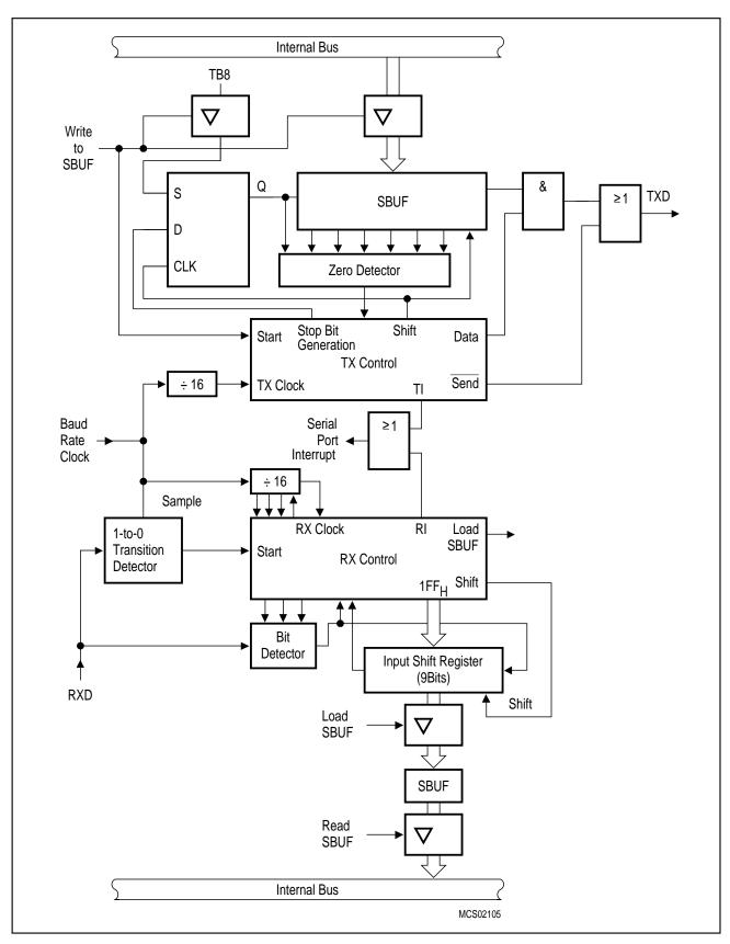
Figure 6-35 Serial Interface, Mode 2 and 3, Functional Diagram
