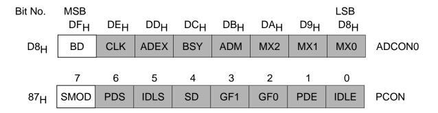
The shaded bits are not used in controlling the serial port baud rate.
