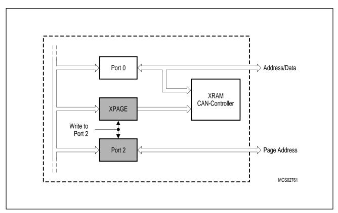
Figure 3-2 Write Page Address to Port 2
