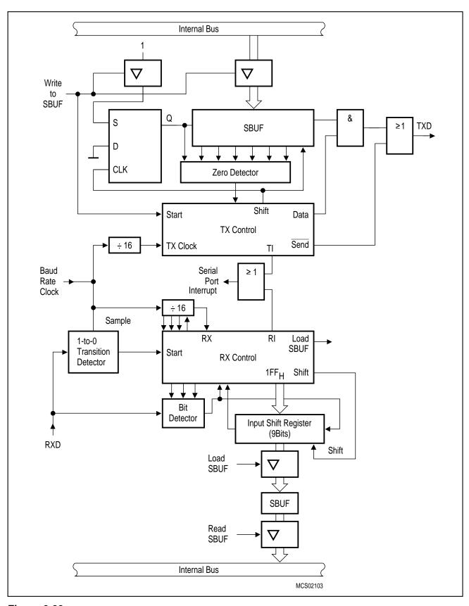
Figure 6-33 Serial Interface, Mode 1, Functional Diagram
