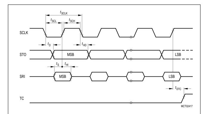
Notes: Shown is the data/clock relationship for CPOL=CPHA=1. The timing diagram is valid for the other cases accordingly.
