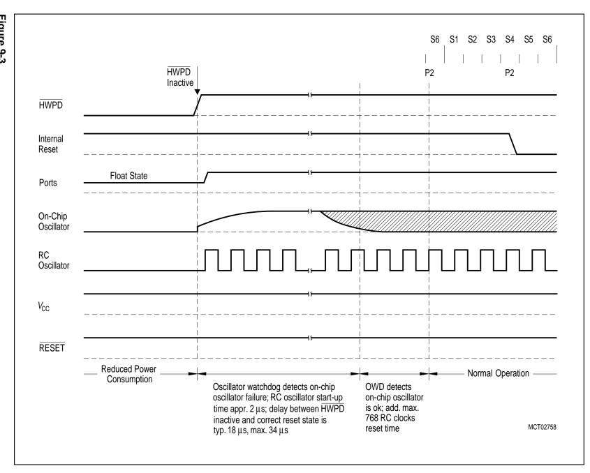
Timing Diagram of Hardware Power Down Mode, HWPD-Pin is active for only one Cycle
