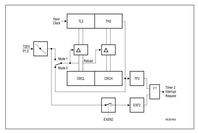
Figure 6-20 Timer 2 in Reload Mode
