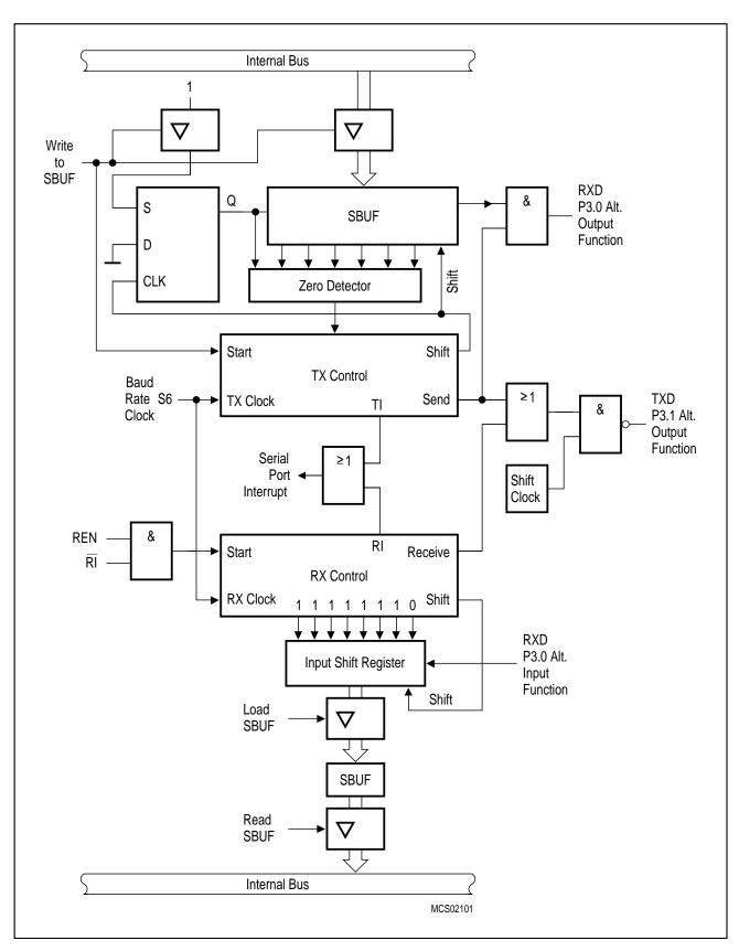
Figure 6-31 Serial Interface, Mode 0, Functional Diagram
