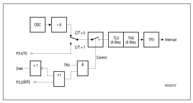
Figure 6-16 Timer/Counter 0, Mode 1: 16-Bit Timer/Counter
