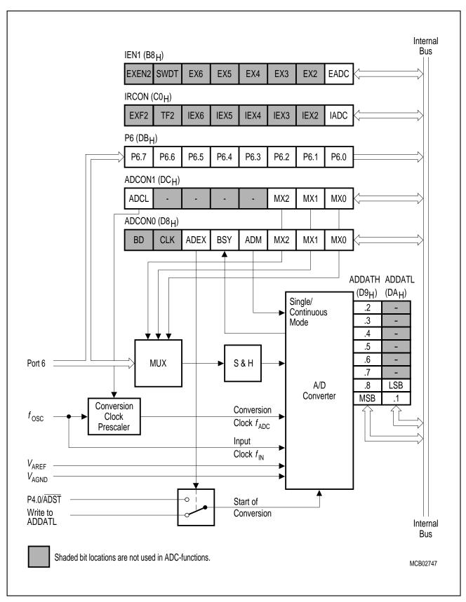
Figure 6-52 Block Diagram of the A/D Converter
