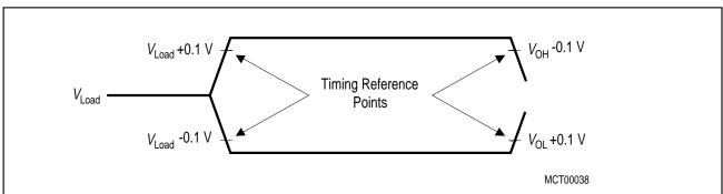
For timing purposes a port pin is no longer floating when a 100 mV change from load voltage occurs and begins to float when a 100 mV change from the loaded  $V_{\rm OH}/V_{\rm OL}$  level occurs.  $I_{\rm OL}/I_{\rm OH} \ge \pm 20$  mA
