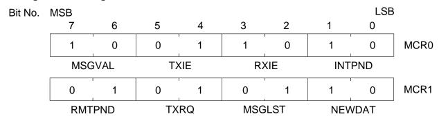
To process the message the microcontroller should clear IntPnd, clear NewDat, process the data, and check that NewDat is still clear. If not, it should repeat the process again. To send a remote frame to request the data, the microcontroller simply needs to set the TXRQ bit. This bit will be cleared by the CAN controller, once the remote frame has been sent or if the data is received before the CAN controller could transmit the remote frame.
