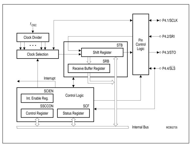
Figure 6-37 SSC Block Diagram
