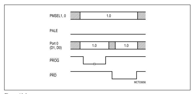
Figure 10-6 Write/Read Lock Bit Waveform
